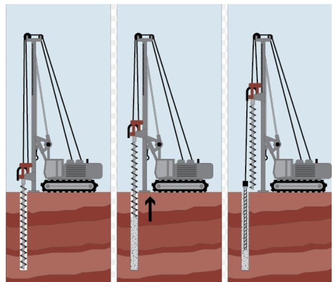
Secant piled walls are formed by constructing reinforced concrete piles that interlock. First a guide wall is constructed to ensure the secant piles are placed correctly. A series of primary piles are installed, then secondary piles, reinforced with high strength concrete and steel, overlap the primary piles. To do this we will require:
